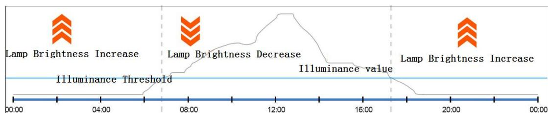
Collect the illuminance of the working surface: when the collected illuminance value is greater than the illuminance threshold, the system decreased the lamp brightness until the collected illuminance value is close to the illuminance threshold; when the collected illuminance value is less than the illuminance threshold, the system increased lamp brightness until the collected illuminance value close to the illuminance threshold.
