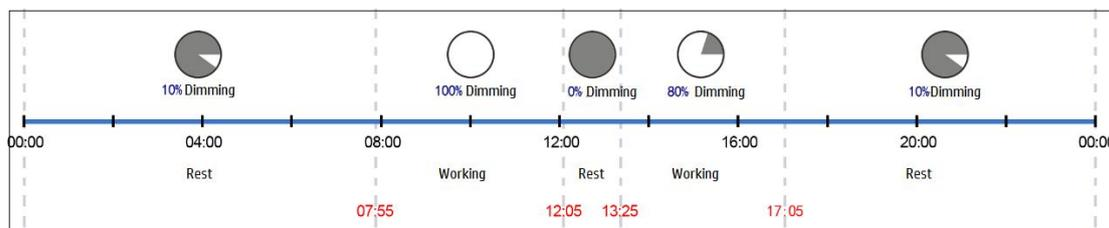
The **Timetable Control Scheme** is that the user sets the working hours of the day according to the Lighting Needs, and sets the illuminance value of the lamps during the working hours at the same time.
