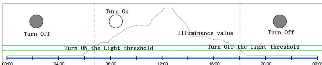
Collect the illuminance of natural light, when the collected illuminance value is greater than the light-on threshold, the system turns on the light; when the collected illuminance value is less than the light-off threshold, the system turns off the light.
