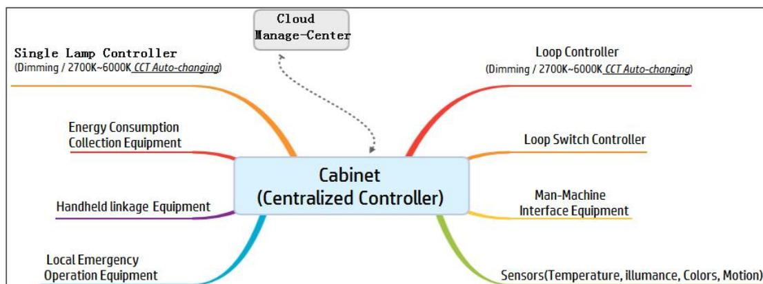
Generally speaking, the system are divided into cloud management center equipment, human-machine interface equipment, local management center equipment, lighting fixture control equipment, sensor equipment, and debugging equipment.
