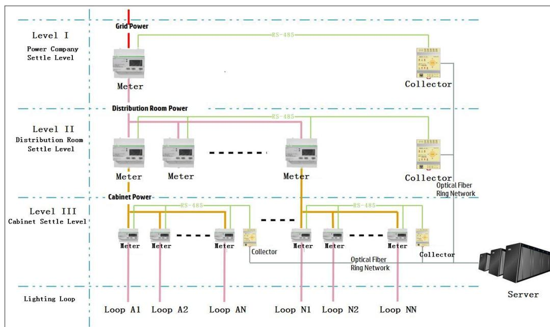
Collect all levels of electrical energy, calculate the line loss of each level, and find abnormalities in the Grid.
